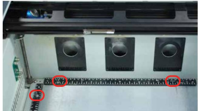
There are three mating pins on the bottom side of the vector grid that fit into the slots in the ruler.
