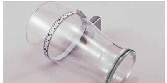
The edge of the black bumper on your Rotary Attachment corresponds to the left edge of your page in CorelDRAW. Set your cylinder on the Rotary Attachment so that it just touches the black bumper. The "top" of a cylinder can be at either end of the Rotary Attachment. It is useful to visualize the orientation of the cylinder when it is being engraved, as is shown in the screen shot on the right.
