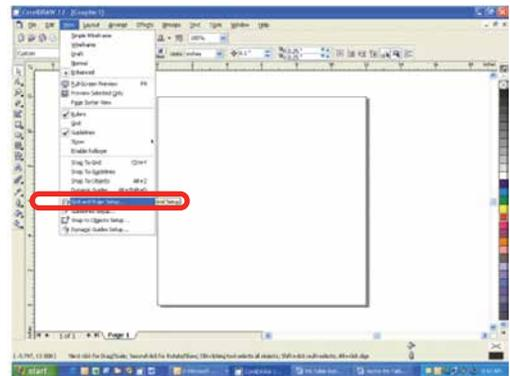
Set the Frequency to 1.0 per inch (both Horizontal and Vertical) and put a check mark in the Show grid box. Click **OK**. Your Corel page now shows a grid pattern that matches the grid of the Pin Table.
